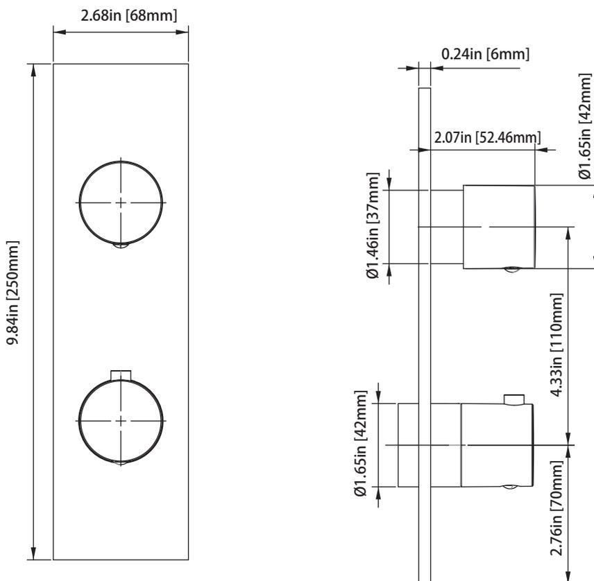
TVH.2717F | 3/4" Thermostatic Valve With 2-Way Diverter & Integrated Volume Control Page 1 of 2
