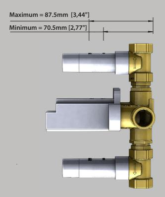
The distance between back of the valve to the finished tile surface should be between 2.77" and 3.44" inches.
