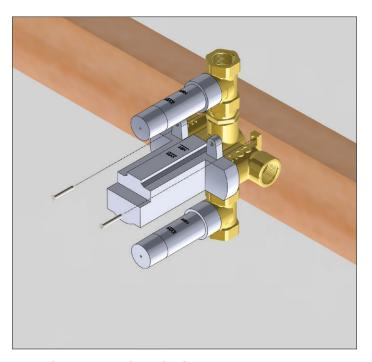
Fix Valve on wooden plank
