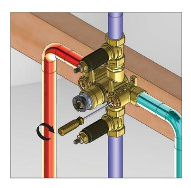
Turn Clock-wise 7 times to stop water flow.
