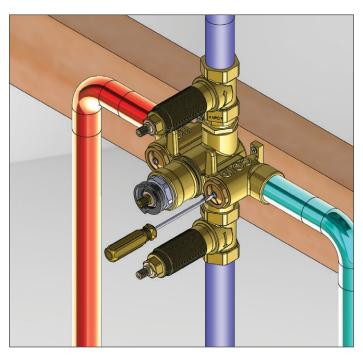
In order to remove the supply stops do not twist the screw in the middle of the supply stop
