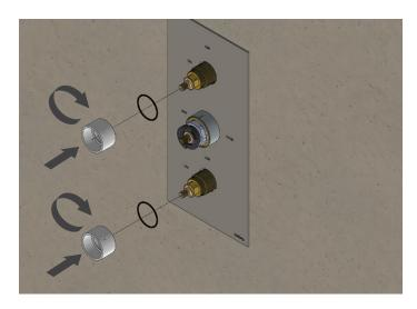
Insert adapter base and tighten
