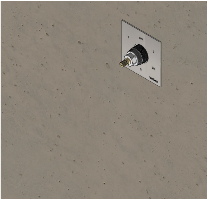
Align Trim plate till it is straight
