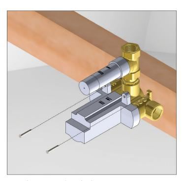
Fix Valve on wooden plank
