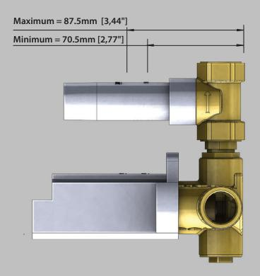
The distance between back of the valve to the finished tile surface should be between 2.77" and 3.44" inches.
