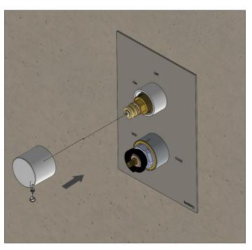
Insert diverter handle. Tighten hex screw & insert cover button. Make sure the diverter is set to the "OFF" marking before your begin
