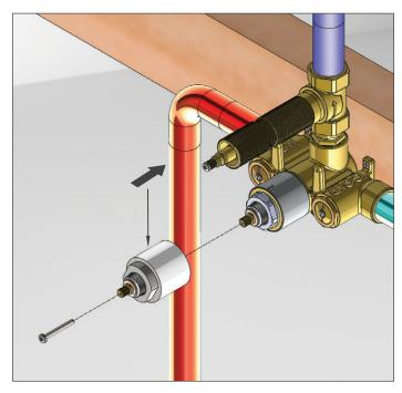
Install temperature extension piece as shown above. Tighten Screw
