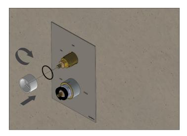
Insert adaptor base and tighten
