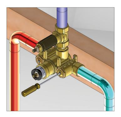
Turn Clock-wise 7 times to stop water flow.
