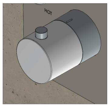
The button on the temperature handle is an anti scald feature. In order to rotate the handle further to "HOT" the button must be pressed
