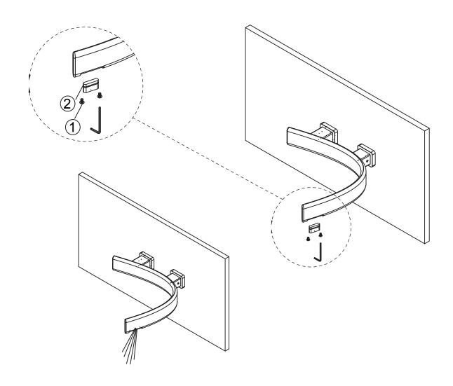
H) After installation is complete, loosen the set screw (1) with a 1.5mm allen key and then remove the aerator (2) with aerator wrench.
