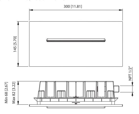
Valve Box should be within 7mm [0.275"] of finished wall
