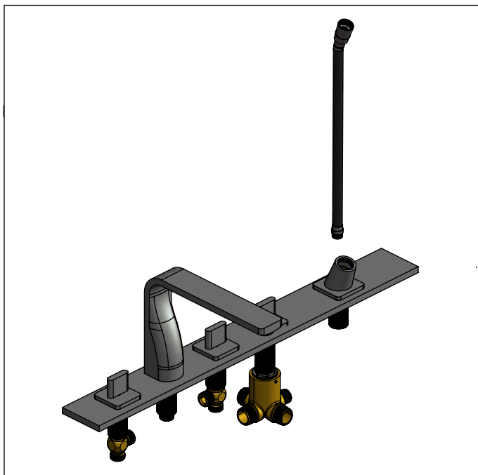
Drop hose down through deck hole
