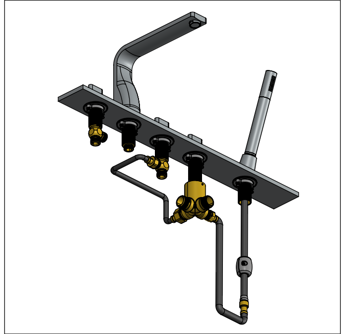
Connect cold side to diverter valve
