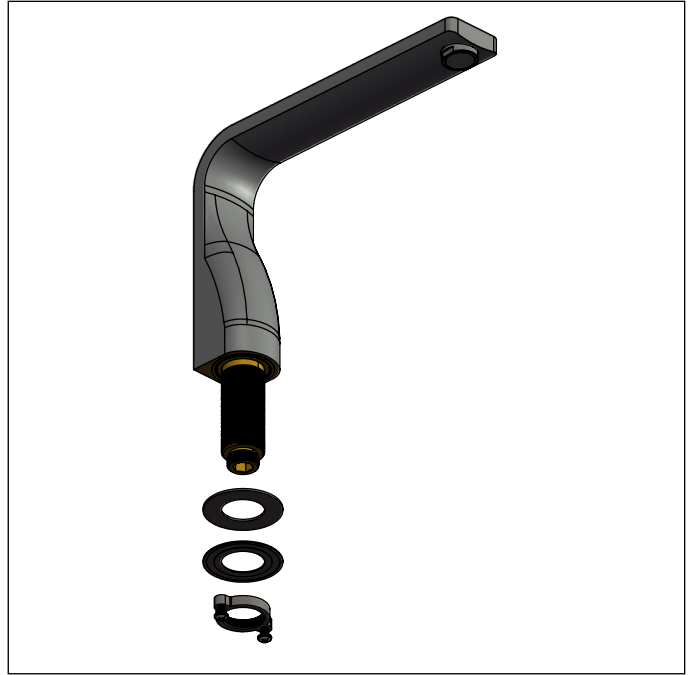
Remove components from cartridge
