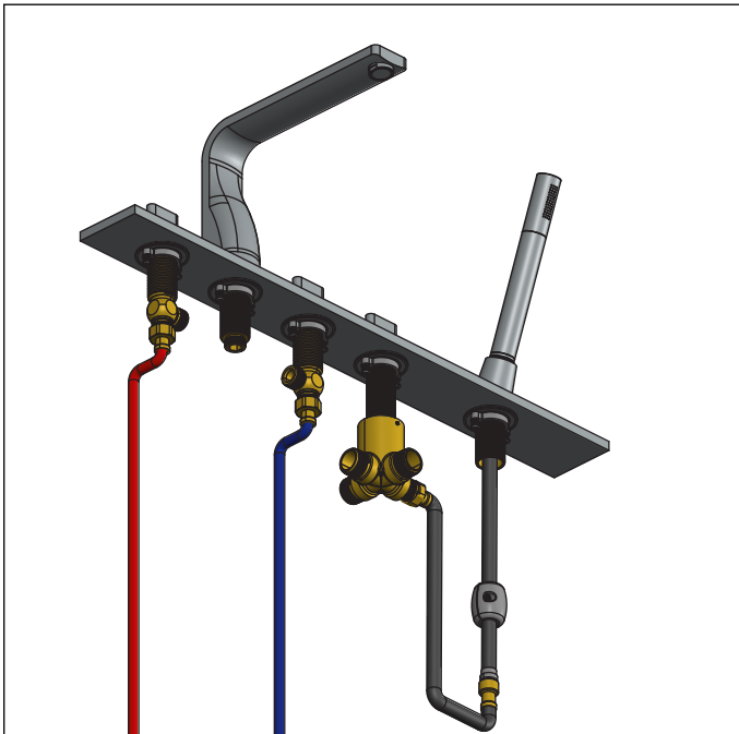
Connect Hot & Cold-Side Connection
