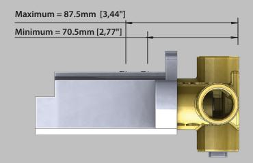
The distance between back of the valve to the finished tile surface should be between 2.77" and 3.44" inches.
