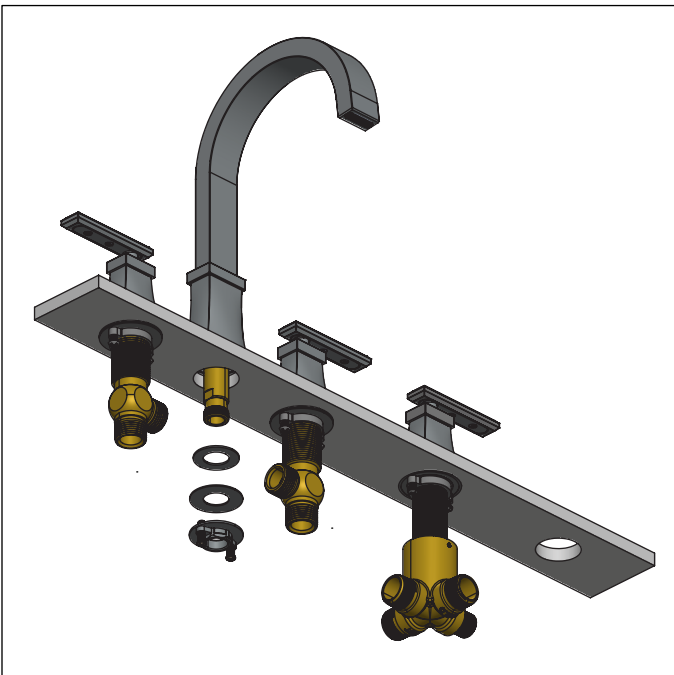
Insert spout into deck hole, then insert washers and tighten retaining nut
