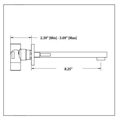
Install a crossbeam at the location where the valve will be installed. The distance between back of the valve to the ÿnished tile surface should be between 2.39" and 3.09".
