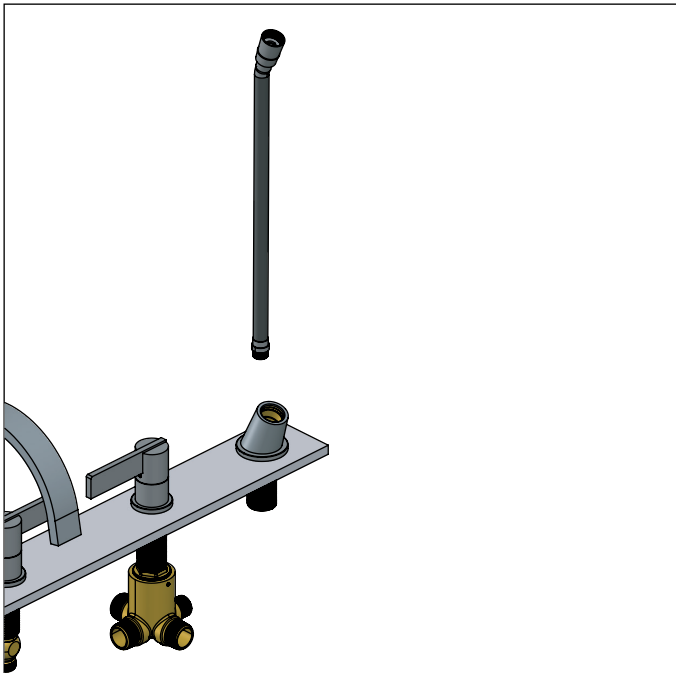
Drop hose down through deck hole
