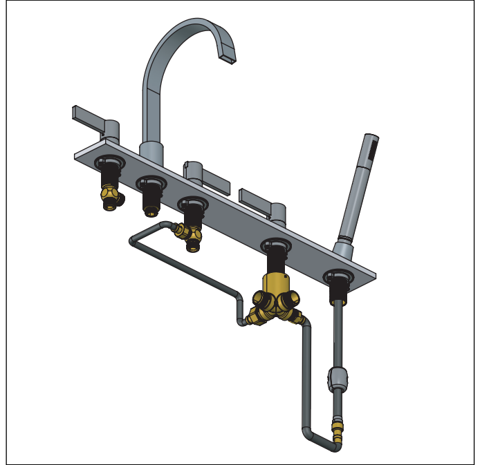
Connect cold side to diverter valve
