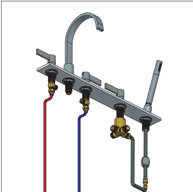
Connect hot & cold-side connection
