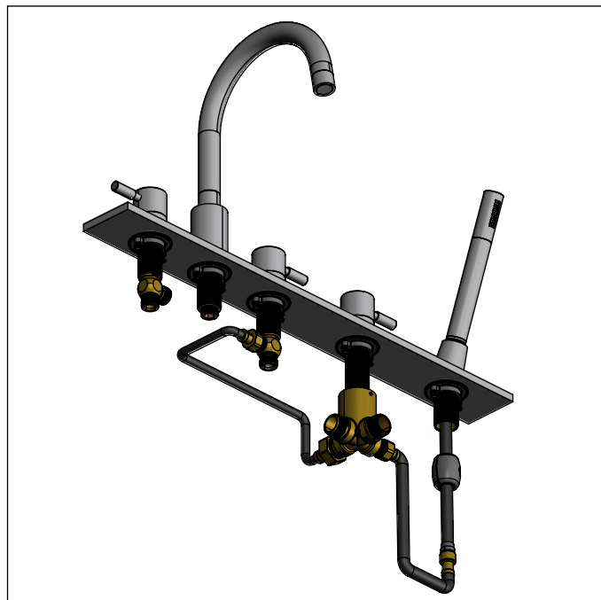
Connect cold side to diverter valve
