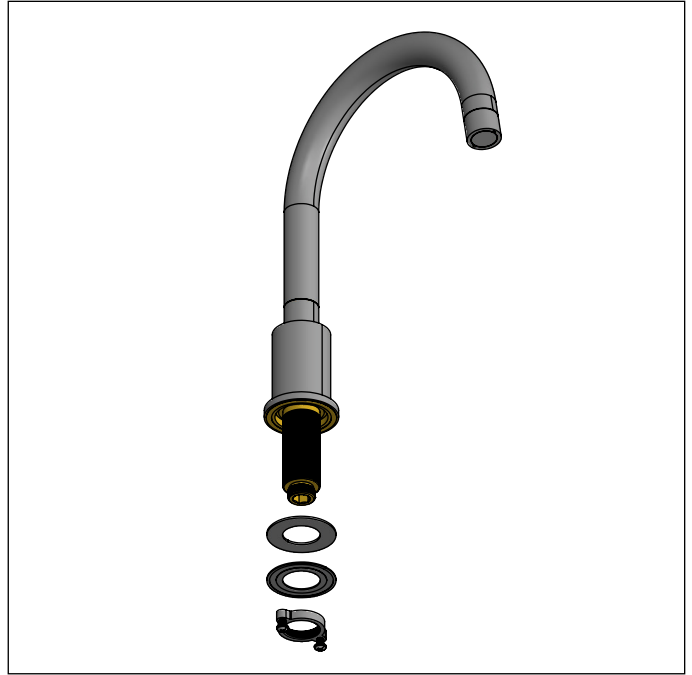
Remove components from bottom of spout.
