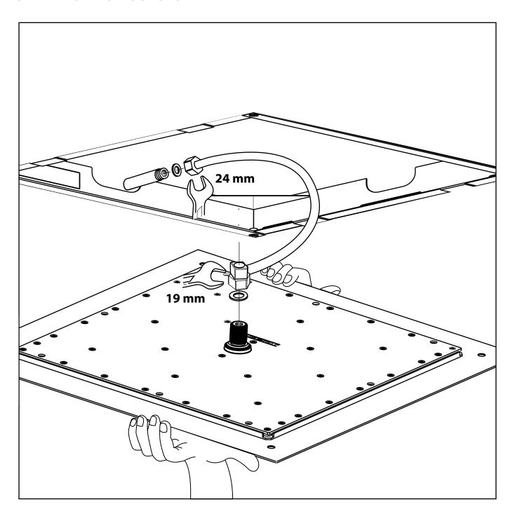
Install water supply hose and tighten. Check For leaks. Then align shower head trim flush to the ceiling and ensure the 4 holes on the edge of the trim align with the mouting box.
